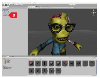
The head has an Adjustment bone (HeadAdj), which serves as an empty slot for addons (04). Other attachment points such as the Hands and Spine have adjustment bones as well.
